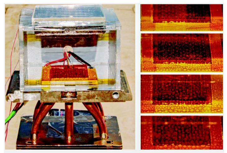
A MOF developed jointly by researchers at MIT and UC Berkeley extracts water vapor from air. As shown on the right, water droplets accumulate over time as the temperature inside the container rises from exposure to the sun.
